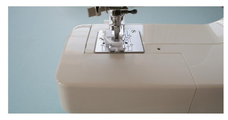
3. Change the setting of your machine accordingly. On' the buttonholeoption, select the matching stitching length and width.
