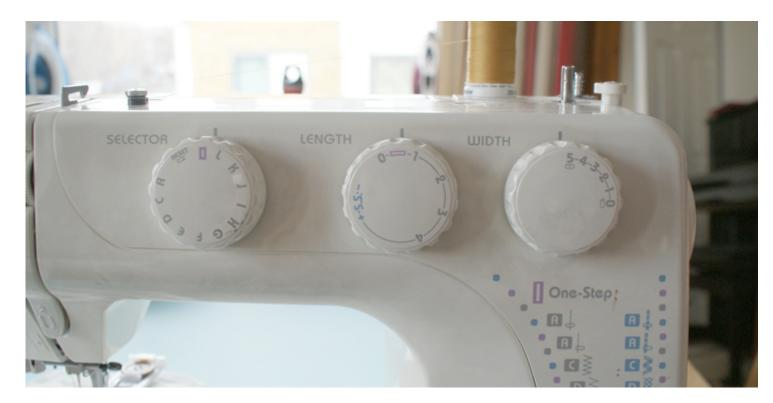
4. Place a piece of scrap fabric under the foot and turn the handwheel slowly towards you with your right hand until the needle goes down and continue turning the handwheel until the take-up lever is at its highest position.
