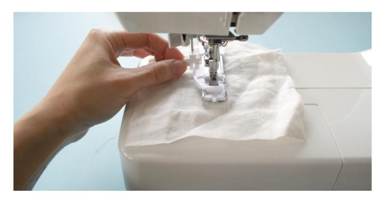
9. Sew slowly and stop the machine when a buttonhole is complete.
