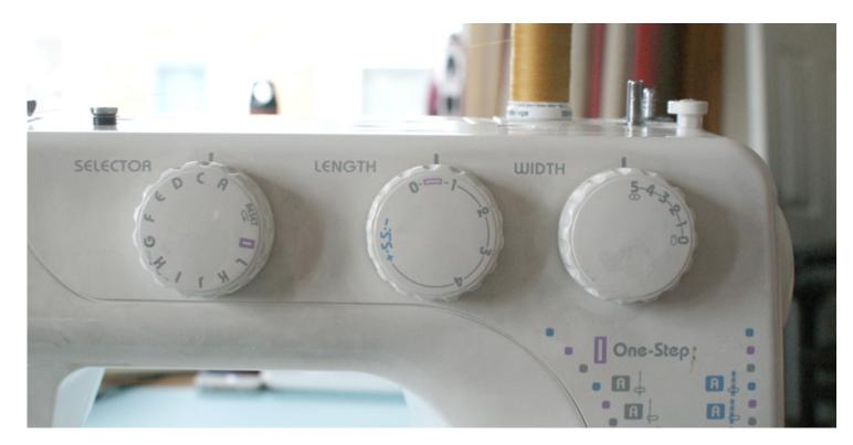
2. Place your fabric under the general sewing foot and lower the needle into the left side of the buttonhole mark.
